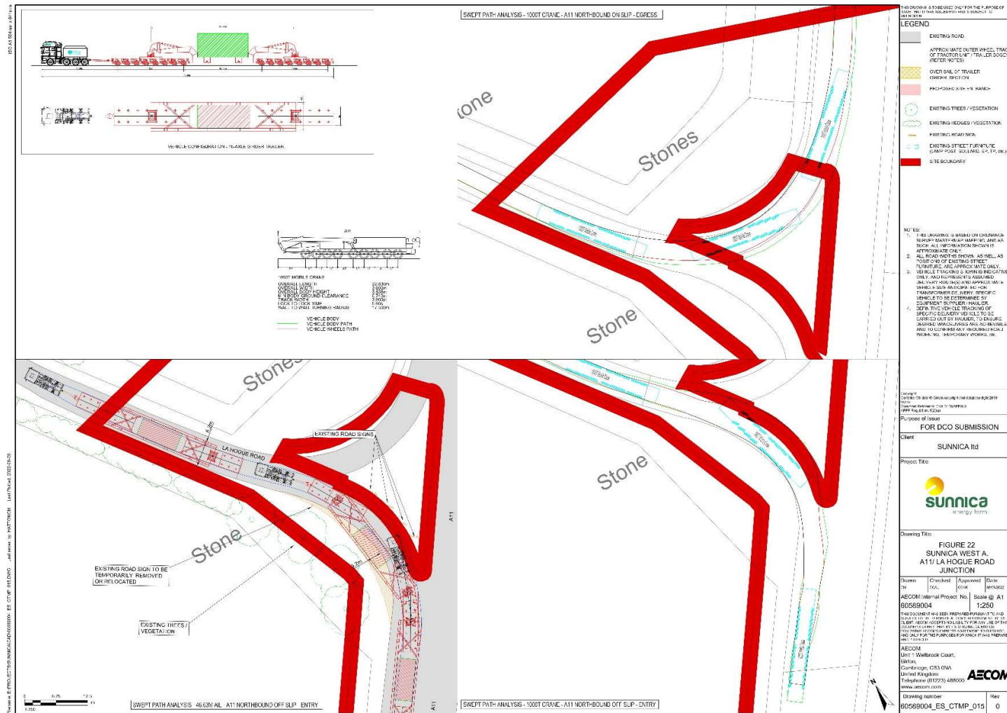
Figure 22: Swept Path Analysis – 1000T Crane and 46.63m AIL – A11 / La Hogue Road Junction
