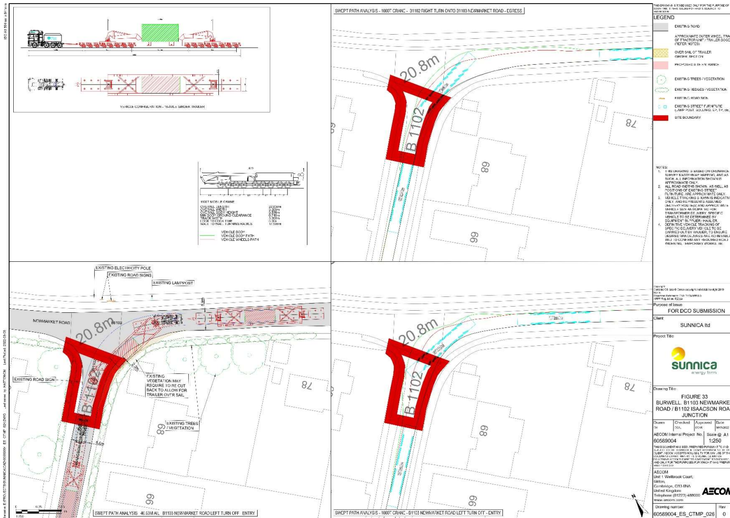
Figure 33: Swept Path Analysis – 1000T Crane and 46.63m AIL – B1103 Newmarket Road / B1102 Isaacson Road Junction
